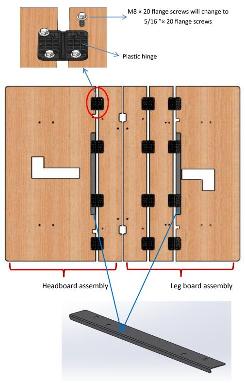
1.8mm Strengthen angle iron Only the bed type of QUEEN and KING has this strengthen angle iron.
